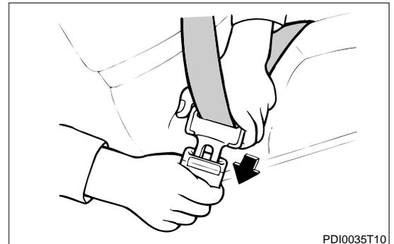
(2) Check that there is no binding while the belt is pulled out or retracted.
