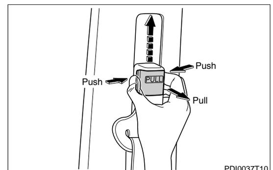
4. Check that the belt is locked securely when hard braking is applied.
