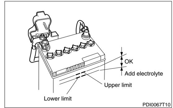
2. Check the battery charging state, based on the specific gravity or the voltage.
