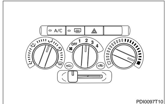
2. Check that the outlet port air changes according to the dial position of the air outlet control dial.
