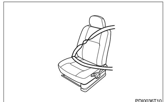
3. Check that the adjustable shoulder anchor can function smoothly and can be locked securely.
