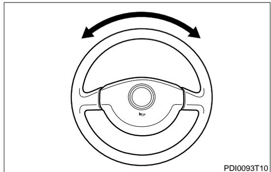
2. When the vehicle is running straight on a flat road, check that the steering wheel directs straight.
