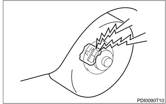
2. Check the exhaust brake. (for diesel engine)
