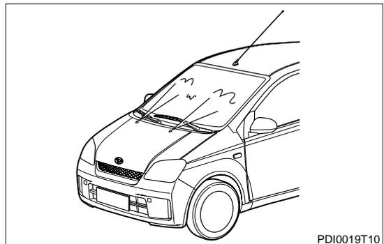
2. Check the wiper for proper operation (intermittent, low speed, high speed, demist).
