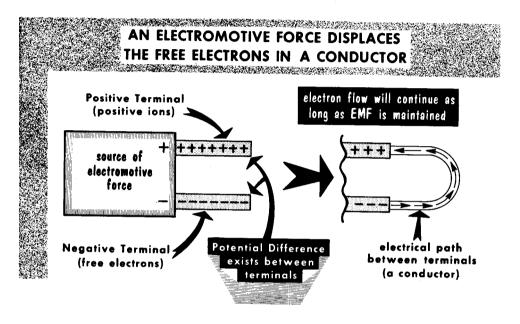
A source of electromotive force can be described as a device in which electrons are forcibly separated from atoms. This creates free electrons and atoms shy electrons or positive ions. The conventional cell or battery used in flashlights and portable radio receivers is an example of sources of electrical pressure or electromotive force. There are other sources about which you will study later.
