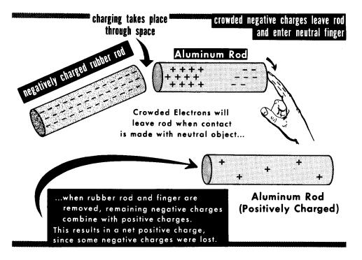
If the charging body had been a positively-charged glass rod, the metal would have had a shortage of free electrons at the end farthest from the glass rod. The positively-charged atoms at this end would pull electrons from the finger that touched the metal. Removing the charged glass rod from the vicinity of the metal would then leave the metal with more free electrons than positively-charged atoms -- or a net negative charge.
