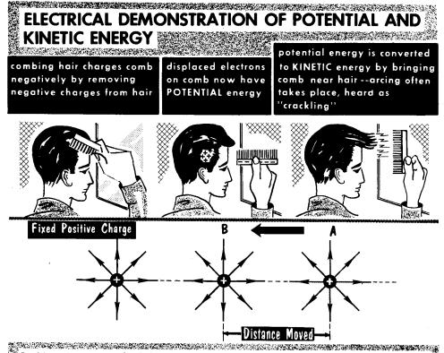
Positive charge at point B has potential equal to Work Done in moving it from point A to point B in opposition to repulsive force of fixed positive charge.
