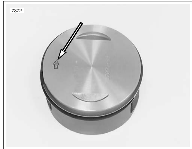
Figure 3-29. Piston Installation Arrow
