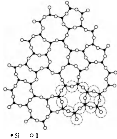
FIGURE 3. Two-dimensional diagram of a random \text{SiO}_2 network. (The fourth bonds of the Si project upward or downward from the plane of the illustration; the actual relative surface area requirement of the oxygens is indicated by dashed lines on the lower right.)
