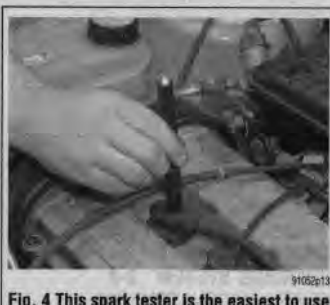
Fig. 4 This spark tester is the easiest to use just place it on a plug wire and the bulb voltage is detected and the bulb on the top will flash with each pulse
