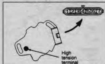
Fig. 12 Distributor connector pins and location—3.5L engine
