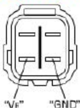
Fig. 25: Identifying HO2S Heater Courtesy of SUZUKI OF AMERICA CORP.
