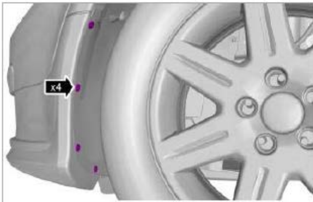
Fig. 2: Identifying Bumper Screws On Inner Front Fender
