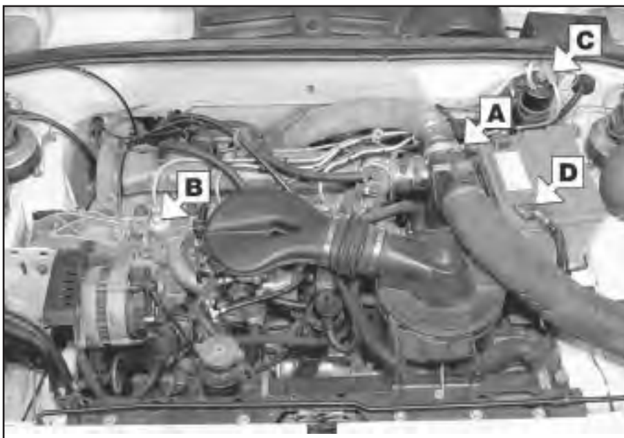
D Check the security and condition of the battery connections.
