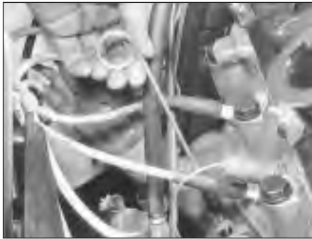
2.2 Withdrawing engine oil dipstick (1116 cc)
