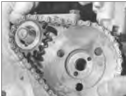
6.13A Fitting the sprockets and timing chain
