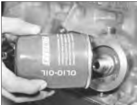
2.8 Screwing on the oil filter (903 cc)
