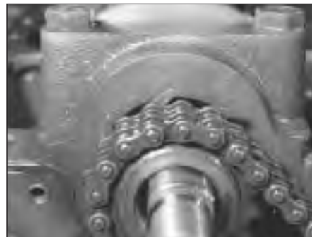
6.13C Self-tensioning links on inside of chain
