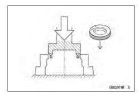
Apply specified grease to the lip of seal before installing the seal.
