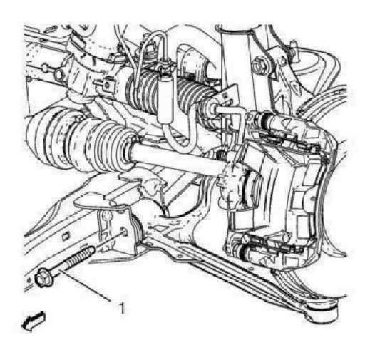
6. Remove and DISCARD the front lower control arm nut and bolt (1).
