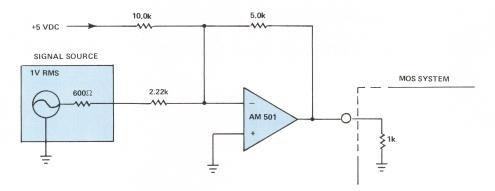
**Problem 1.—**A sinewave source needs to be clocked into an MOS system. The amplitude is insufficient (one volt RMS behind  $600 \Omega$ ) and the DC level is wrong (centered at ground). The signal has to swing between zero and at least five volts minus.
