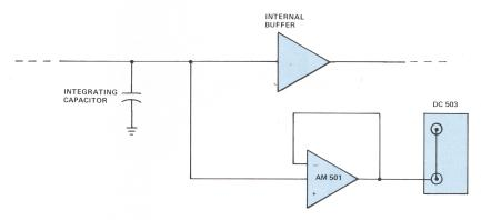
Problem 2. You want to connect the signal on an integrating capacitor to a time-interval meter (TIM). The signal amplitude is several volts, and only a few nanoamps of load current can be tolerated; the one megohm input impedance of the TIM is too low. The circuit under test has an internal buffer, but it shifts the DC level to an unsuitable value. Capacitive coupling will introduce signal aberration or excessive load current.
