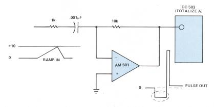
**Problem 3.** A system generates ramps at random intervals. The ramps are of uniform amplitude, but are of two different durations. You want to count the number of fast ramps only, which occur in one hour. Both ramps have a 10 V amplitude; the slow ramp has a duration of  $50 \mu \text{sec}$  and the fast ramp lasts  $10 \mu \text{sec}$ . Solution—Using the AM 501, differentiate the ramps so that only the fast ramp generates an output voltage
