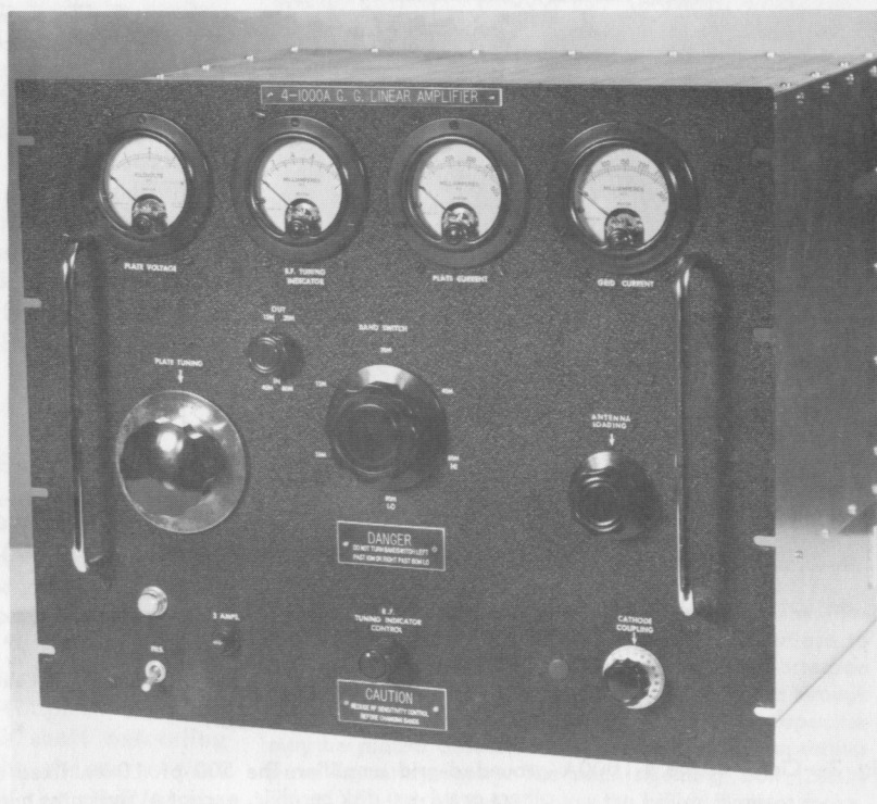
Fig. 1—K9LKA's kilowatt 4-1000A grounded-grid amplifier. Meters across the top of the panel are, from left to right, for plate voltage, relative r.f. output, plate current and grid current. The band-switch control is in the center, flanked by the plate tuning control and capacitor switch S_2 on the left, and the output loading control on the right. Along the bottom are the filament switch, panel lamp and fuse; r.f.-indicator sensitivity control, and the input tuning control.
