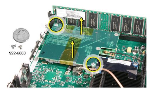
14. Turn over the mezzanine board. With a jeweler's #0 Phillips screwdriver remove the two screws on the Bluetooth board. Pull the Bluetooth board off the connector on the mezzanine board.
