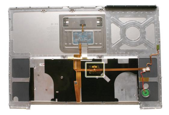
3. Peel off any tape to gain access to the connector.
