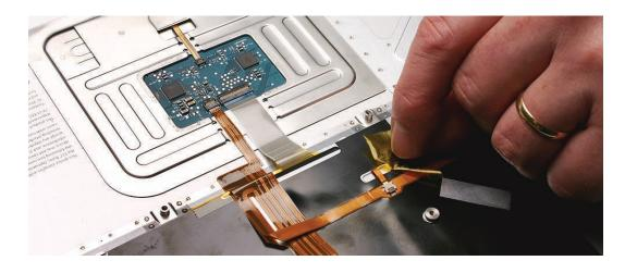
4. Locate the protective cover over flex cable connectors. This will not be removed, but released only half way around to access the large flex cable connector.
