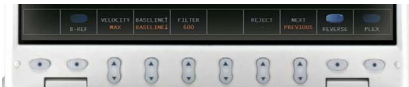
Figure 1: Example of a reconfigurable GUI menu on the lower part of the main screen and buttons and toggles to operate it.
