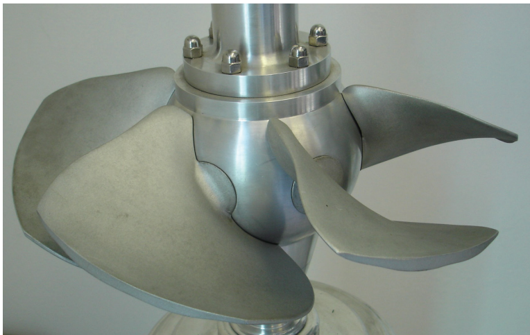
FIGURE 2.4 Model of hydroelectric turbine.
