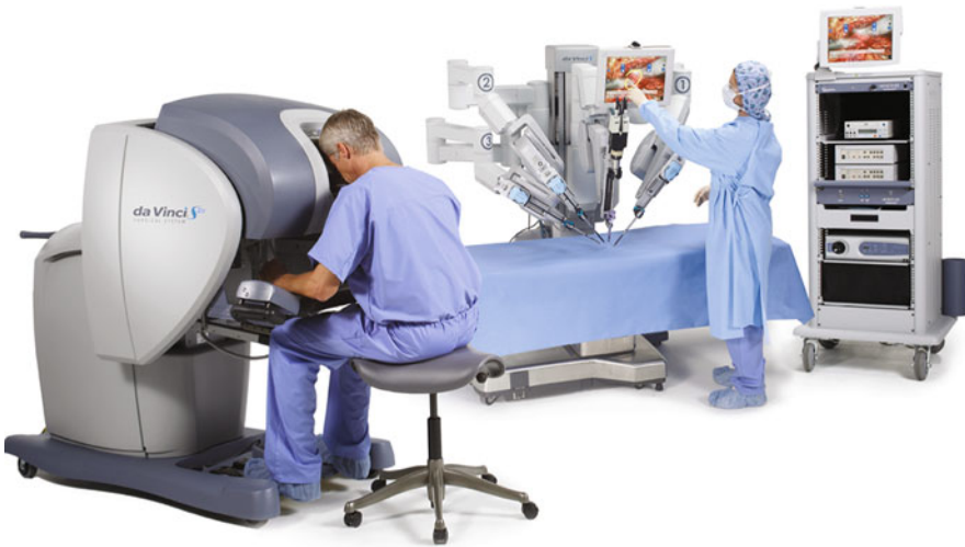
Fig. 1.18: Replicating the surgeon's hand motion with a robotic interface mounted to the patient couch (da Vinci Surgical System, ©2015 Intuitive Surgical, Inc.)
