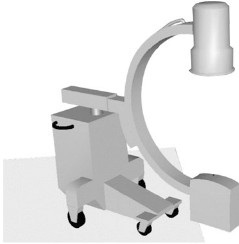
Fig. 1.9: C-arm X-ray imaging. A C-shaped structure carries an X-ray source and an X-ray detector. The C is mounted to a jointed mechanism with five joints [2]
