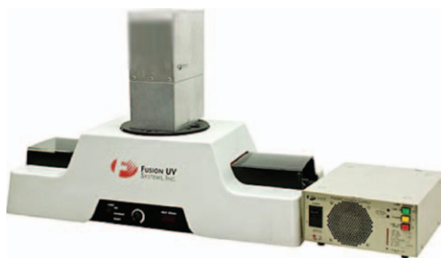
Figure 2.2 FUSION LC-6B Benchtop Conveyor UV Curing System ( http://www.caeonline.com/listing/product/182588/axcelis-fusion-lc-6b ).
