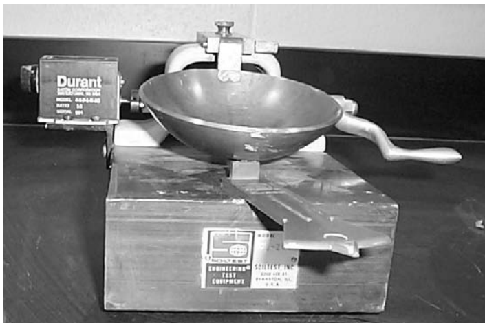
Fig. 4.2— Checking the drop height of the cup using the calibration tab on the grooving tool.
