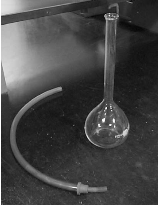
Fig. 3.1—Etched flask along with stopper and tubing for connecting to vacuum source.
