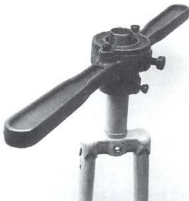
Figure 8. Steerer tube thread cutting
