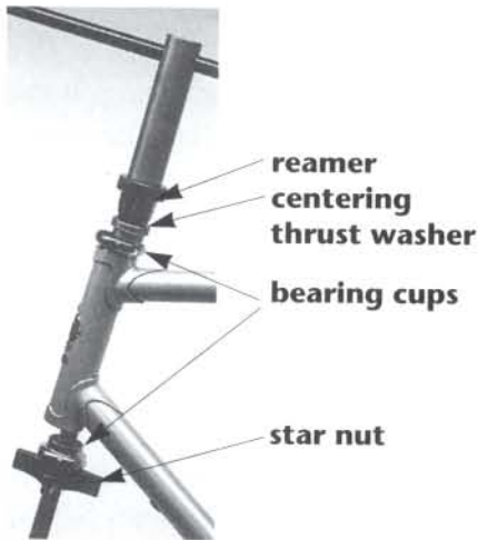
Figure 6. Head cup press assembly
