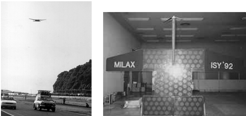
Figure 1.7. The MILAX project airplane experiment showing the model airplane and the phased array used in Japan in 1992
