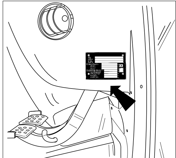
Fig. 2 - Type of tractor and chassis and cab number (on dashboard lower panel).
