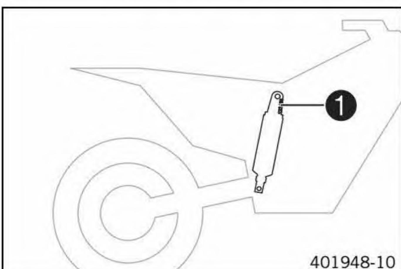
The shock absorber part number **1** is stamped on the top of the shock absorber above the adjusting ring towards the engine side.
